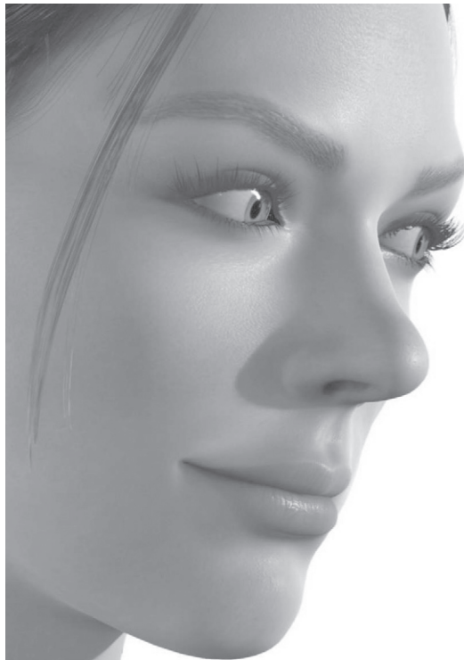
FIGURE C.3.2 GPU-rendered image. To give the skin visual depth and translucency, the pixel shader program models three separate skin layers, each with unique subsurface scattering behavior. It executes 1400 instructions to render the red, green, blue, and alpha color components of each skin pixel fragment.
